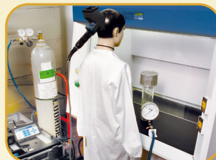
Tracer Gas (SF 6 ) Containment Test
