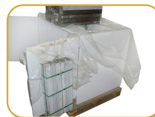
Actual photo during Door Hinge Test
